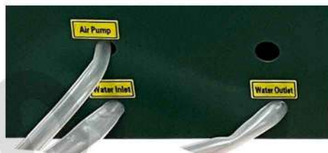
AIR PUMP | WATER INLET | WATER OUTLET
